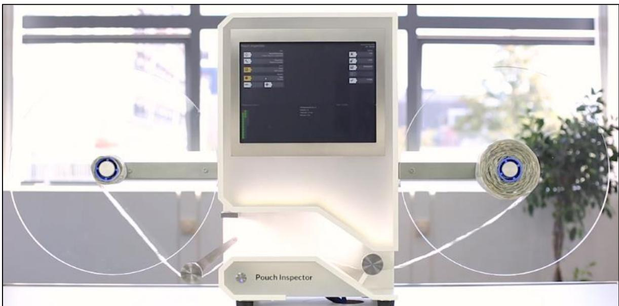
It's also possible to swipe the pouch strips through the machine manually without using the left arm. Swipe it through with a maximum speed of 5 pouches per second and all the pouches will be scanned.
